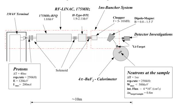
Figure 1: Sketch of FRANZ.  $\Delta T$  is the length of one macro bunch. The distance between the <sup>7</sup>Li-target and the sample is given by 0.8m. The single bending magnet in this figure is just a symbol for a more complicated bending system. (see Fig.2)
