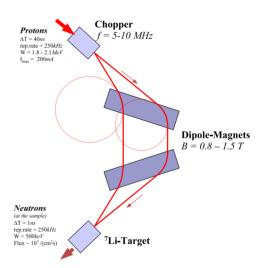
Figure 2: 1ns-Buncher-System. A bending system composed of two skew magnets with spatial non-constant magnet fields would have several advantages, e.g. more paramters in order to manipulate the beam dynamics, in average a greater distance between two bunches and a more compact geometry.
