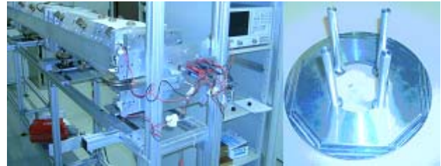
Figure 6: The experimental setup (left) and the stabilizing rods mounted on the coupling plate (right)
