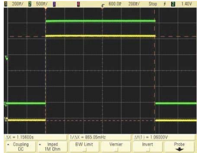
Figure 4: Upper trace is test signal with amplitude of 53mA, and the lower is the output signal having amplitude of 1.06V. The width of pulse is 0.89sec.
