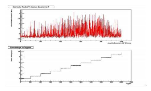
Figure 3: Data taken with the injection seeder turned off. The top plot shows the calorimeter output (arbitrary units) versus the laser spot position at the IP (in microns). The bottom plow is the corresponding piezo scanner voltage (Volts) versus the trigger number (laser shot number).
