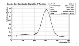
Figure 6: Data analysis of the experiment with injection seeded turned-on. The plot shows shows 11 points, where each point is the averaged calorimeter readout per piezo voltage, versus the movement at the IP (in microns).
