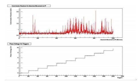
Figure 4: Data taken with injection seeding turned-on. The top plot shows the calorimeter output (arbitrary units) versus the laser spot position at the IP (in microns). The bottom plot shows the corresponding piezo scanner voltage (Volts) versus the trigger number (laser shot number).
