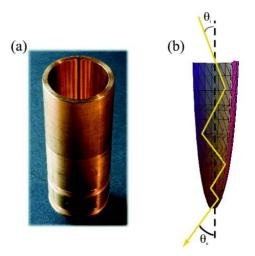
Figure 4: (a) A brass non-imaging light concentrator as used in this experiment, (b) light reflecting through the concentrator.
