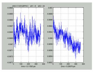
Figure 4: Libera noise in Slow Acquisition mode: Xrms =  $0.11 \mu m$ , Zrms =  $0.25 \mu m$  (360 acquisitions in 180 s).
