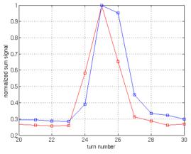
Figure 2: Good beam phase with respect to the MC (red curve) and wrong beam phase (blue curve).
