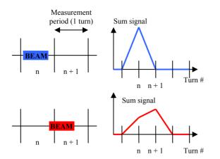
Figure 1: One-turn Sum signals on two BPMs with different phases of the beam with respect to the Machine Clock (MC).
