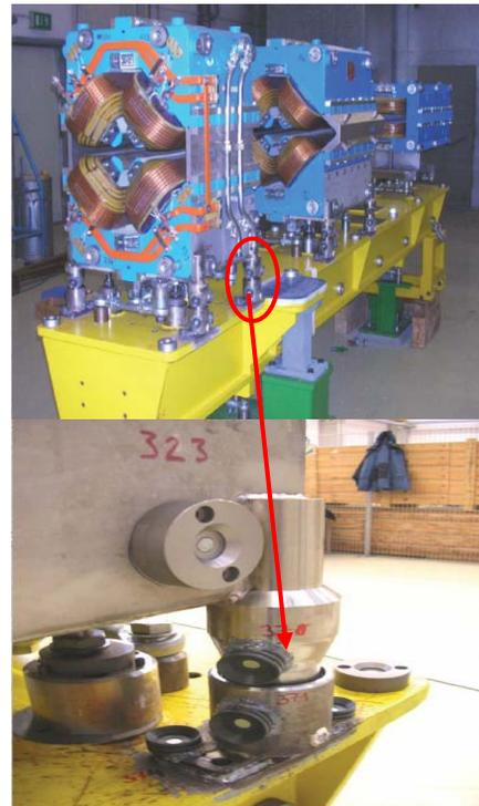
Figure 2: In order to maintain the quality of the alignment of the magnets they are glued to the girder.
