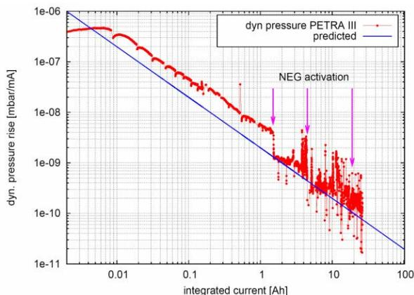
Figure 3: Comparison between expected and measured dynamic pressure rise as a function of integrated current for the test chambers installed in PETRA II.
