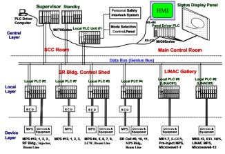
Figure 1: Configuration of MIS.
