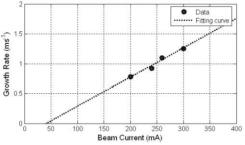
Figure 5: Growth rate of vertical mode #198 as a function of stored beam current. The estimated growth rate is slightly less 2 ms<sup>-1</sup> at 400 mA.
