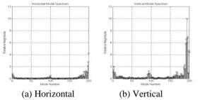
Figure 6: Modal spectrum of the typical 300 mA stored beam.
