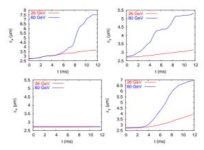
Figure 3: Horizontal (left) and vertical (right) emittance growth due to electron cloud at 26 and 60 GeV/c. Simulation results are shown for a field-free (upper) and a dipole (lower) region.
