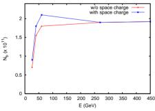
Figure 2: Simulated TMCI threholds at different energies, with and without space charge.
