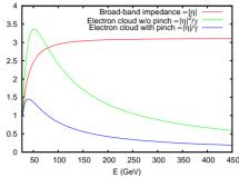
Figure 1: Energy dependence of the TMC and TMC-like instability threholds as theoretically expected. Values are normalized to the 26 GeV/c case.
