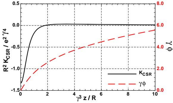
Figure 2:  $K_{\text{CSR}}$  and  $\phi$  as a function of  $z$  for a bend.
