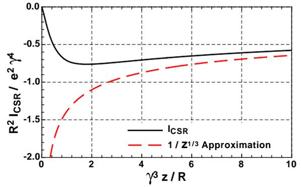
Figure 3:  $I_{\text{CSR}}$  a function of  $z$  for a bend. The dashed line is the large  $z$  approximation as given in Eq. (16).
