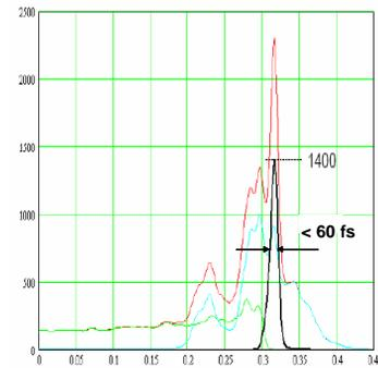
Figure 6: Predicted current distribution in front of the undulator according to beam dynamics calculations.
