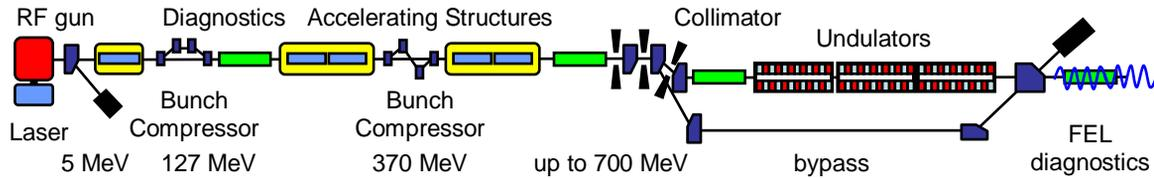
Figure 2: Schematic layout of the *Free-Electron Laser in Hamburg, FLASH* at DESY.
