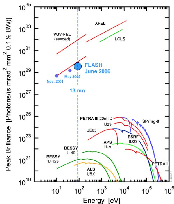
Figure 14. Peak brilliance demonstrated at FLASH (dots), compared with expected values (solid line), with values of some FELs under construction (LCLS) or proposed (European XFEL), and with values of state-of-the-art synchrotron radiation sources.
