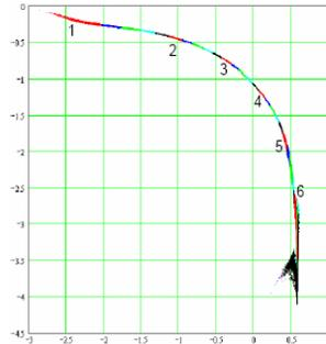
Figure 4: Longitudinal momentum distribution 1 m after the first bunch compressor. The head of the bunch is to the right.
