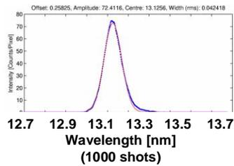
Figure 13. Averaged spectrum of 1000 pulses at FLASH tuned for 1<sup>st</sup> harmonics at 13 nm wavelength.
