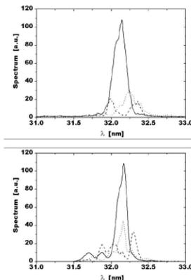
Figure 9. Top: Three different single-shot wavelength spectra of FEL radiation pulses at 32 nm wavelength measured at FLASH. A pulse length of ~25 fs can be inferred from the width of individual spikes in the spectrum [28]. Bottom: Predicted spectrum for three different electron statistics seeds [17]. Note that the number of spikes in the spectrum is in average equal to the number of spikes (coherent wave packets) in the time domain.
