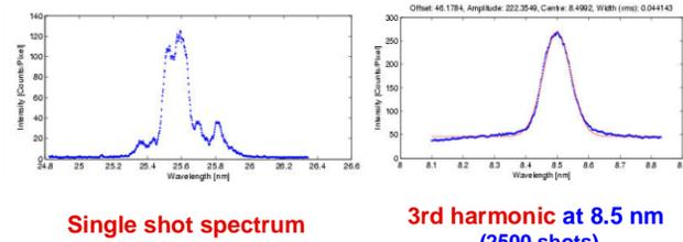
Figure 11. Single shot spectrum at 25 nm wavelength (1<sup>st</sup> harmonics) (left), and corresponding 3<sup>rd</sup> harmonics spectrum (right).
