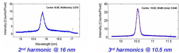
Figure 10. Second and third harmonics spectra averaged over 4000 radiation pulses.
