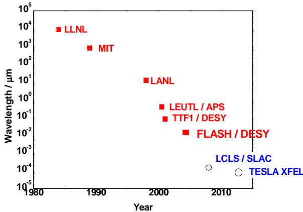
Figure 1: Progress on wavelengths achieved at SASE FELs vs year of 1<sup>st</sup> operation. Red squares: Successful demonstration, in most cases reaching laser saturation; Blue dots: Projects under way.
