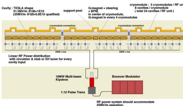
Figure 6: ILC one RF unit installed in the ILCTA
