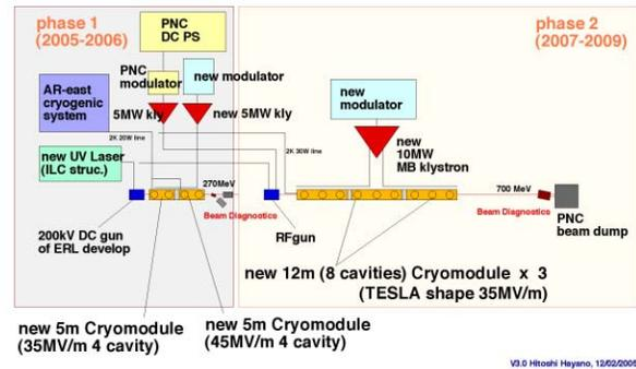
Figure 8: Superconducting Test Facility (STF) Plan in KEK
