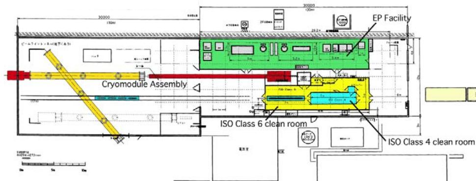
Figure 9: Planed EP, String assembly, and Cryomodule assembly facility on the ground level in the STF building
