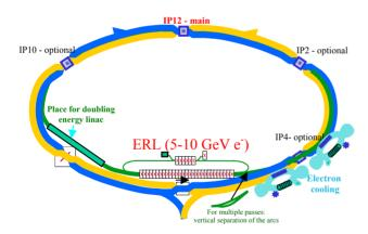
Figure 2: Linac-ring design option of eRHIC uses the energy recovery linac as the electron accelerator.
