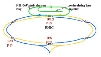
Figure 1: Ring-ring option of the eRHIC uses the electron (or positron) beam from a storage ring for collisions with ions or protons, circulating in RHIC, in one of the RHIC existing interaction points.
