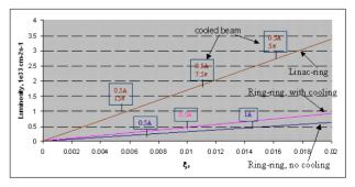
Figure 3: Comparison of the luminosities versus proton beam-beam parameter for the linac-ring and the ring-ring option, with and without the transverse electron cooling of the proton beam. 330 bunches are assumed in the proton ring with 1.e11 proton per bunch. Markers demonstrate the luminosities for the indicated electron
