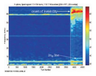
Figure 5: Vertical frequency spectrum vs turn.
