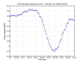
Figure 8: Phase transient of the beam at the onset of the instability.
