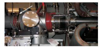
Figure 10: Flange with dislocated gap ring.
