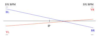
Figure 2: Derivation of the relative offset of the two beams at the IP from BPM measurements taken at the DX separator dipoles.
