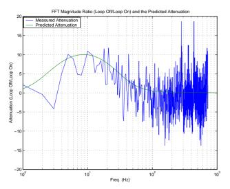
Figure 7: Measured IP orbit offset reduction.
