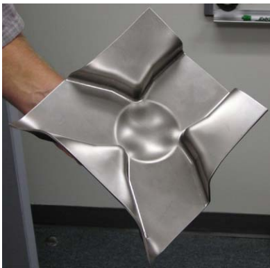
Figure 8. Pressed waveguide end group before trimming.
