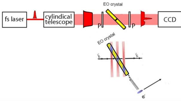
Figure 1: Simplified scheme of the EO spatial decoding. The laser and the field of the bunch are polarized horizontally, parallel to the  $(-1,1,0)$  axis of the GaP crystal. Due to the angle of incident of 45 degree, the position of the polarization variance inside the beam profile is depending on the relative arrival of the optical pulse and the electron bunch at the EO crystal.
