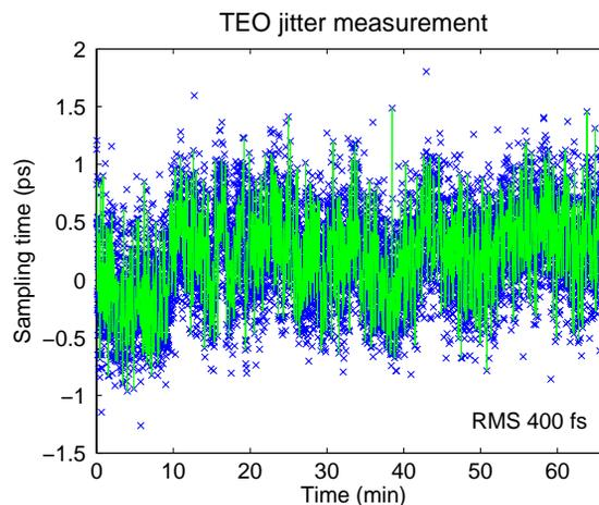
Figure 5: Measurement of the relative arrival time jitter over 60 minutes (data points with interpolated spline function). The RMS jitter is 400 fs.
