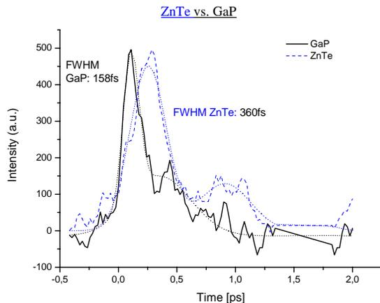
Figure 4: Comparison between the TEO signal with GaP and ZnTe crystal. The temporal position of relative arrival is given by the rising edge. The rise time of the GaP EO signal is 100 fs.
