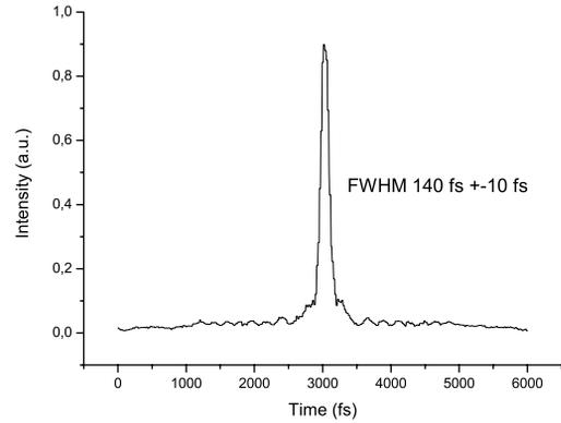
Figure 3: Autocorrelation of recompressed laser pulse at EO crystal. Assuming a Gaussian profile, duration of the laser pulse is 100 fs. The influence of the remaining TOD leads to small oscillations visible in the wings.
