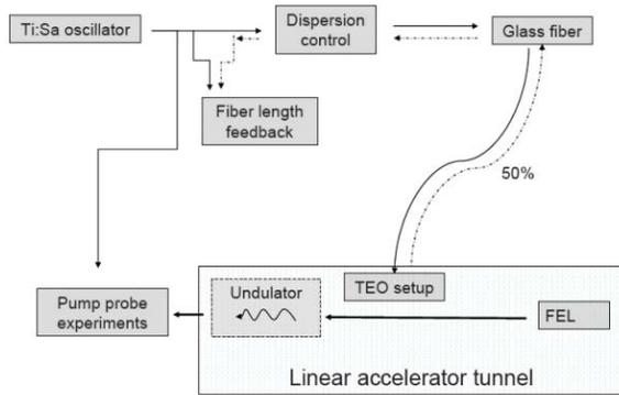
Figure 2: Scheme of the Timing by Electro-Optical Sampling (TEO) experiment.
