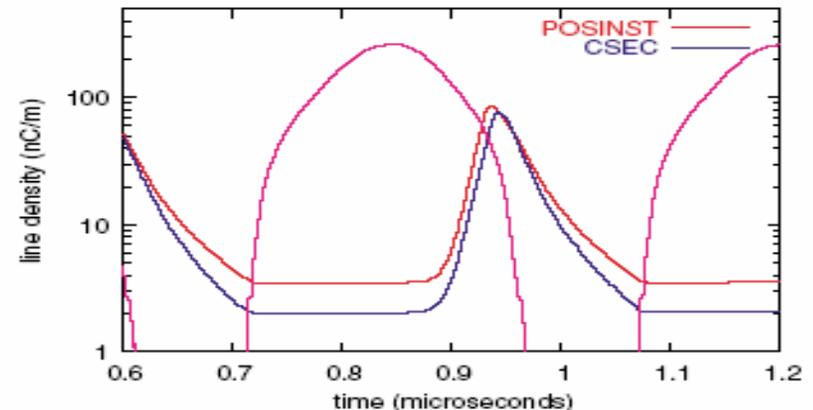
FIG. 6. (Color) Beam line density (purple) and total electron cloud line densities for the PSR obtained with CSEC (blue) and POSINST (red).
