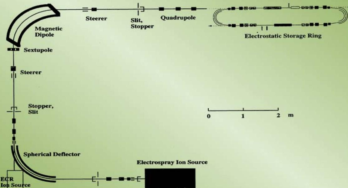
**Layout of the ion sources, the mass-analyzer and the electrostatic storage ring.** D<sub>1</sub> and D<sub>2</sub> are 10° and 160° deflectors, QF and QD the horizontally focusing and defocusing electrostatic quadrupoles, PM-H and PM-V the horizontal and vertical position monitors, RF system and V-ST the vertical steerer.
