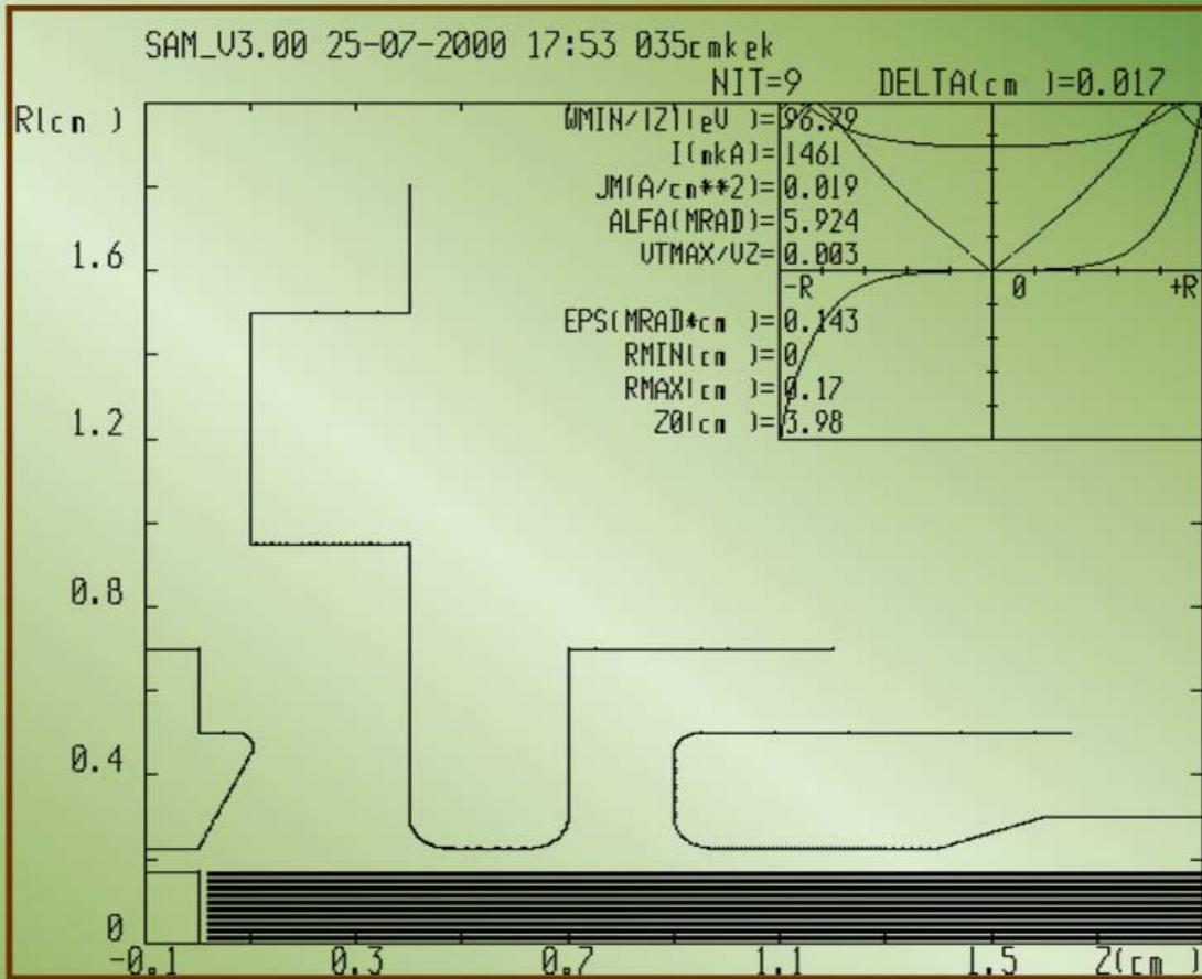
Maximum beam permeance corresponds to a vacuum chamber permeance of  $10 \mu\text{A}/\text{V}^{3/2}$
