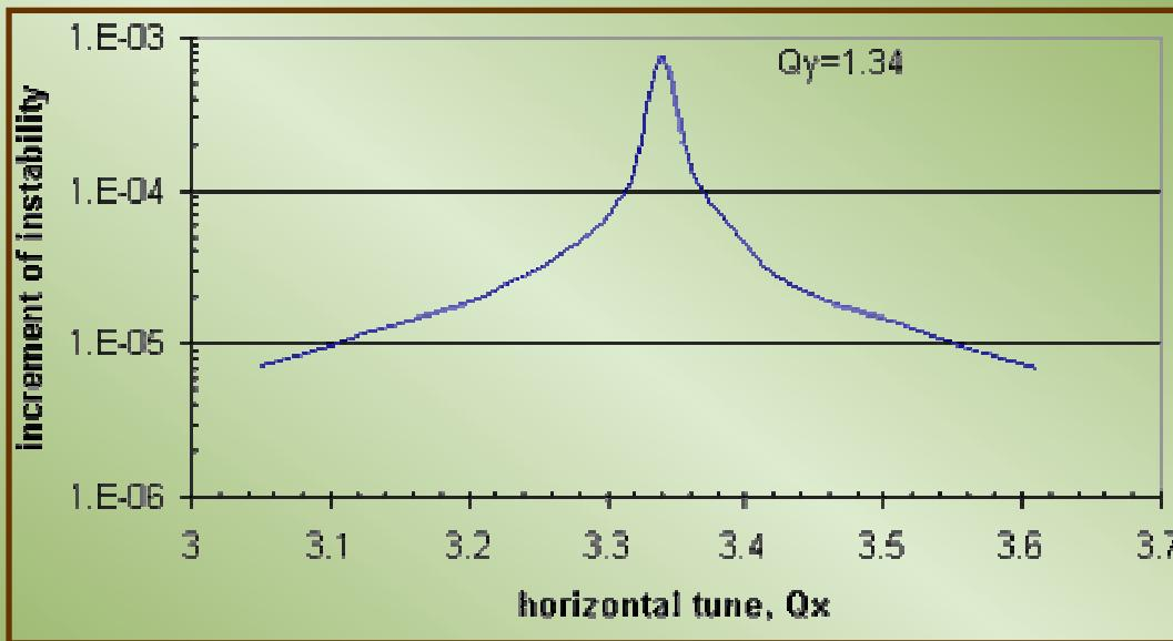
Dependence of the increment on the horizontal tune at  $Q_y=1.34$ ,  $I=0.1$  mA,
