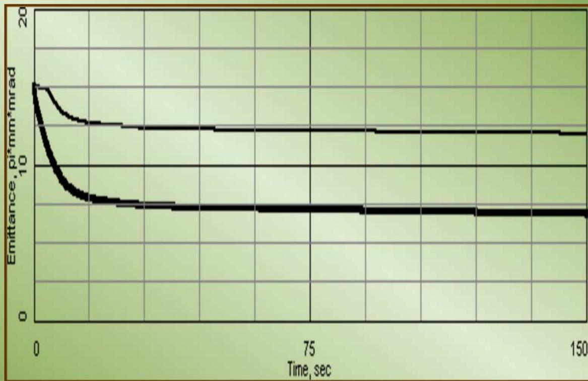
Dependence of ion ( $A=300$ ,  $Z=-2$ ) emittance on the time at the cooler parameters:
