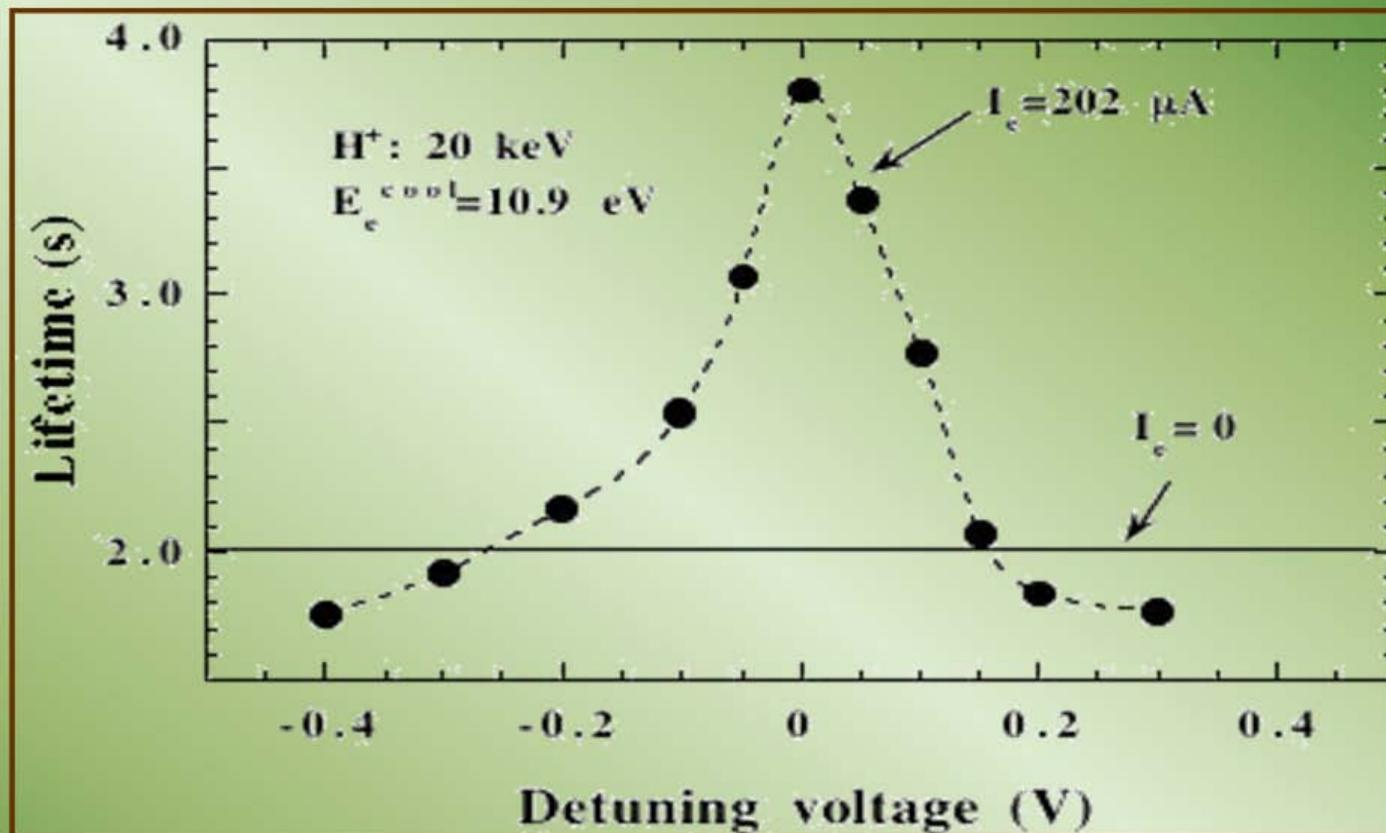
Lifetimes of 20-keV  $\text{H}^+$  beam with and without electron beam as a function of detuning acceleration voltage of electrons. The tuned voltage is 14.5 V.
