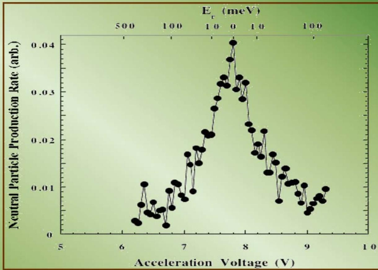
Dissociative recombination rate for  $\text{H}_2^+$  with an energy of 20 keV as a function of the electron acceleration voltage at  $I_e = 60 \mu\text{A}$  and  $B = 30 \text{ G}$ .
