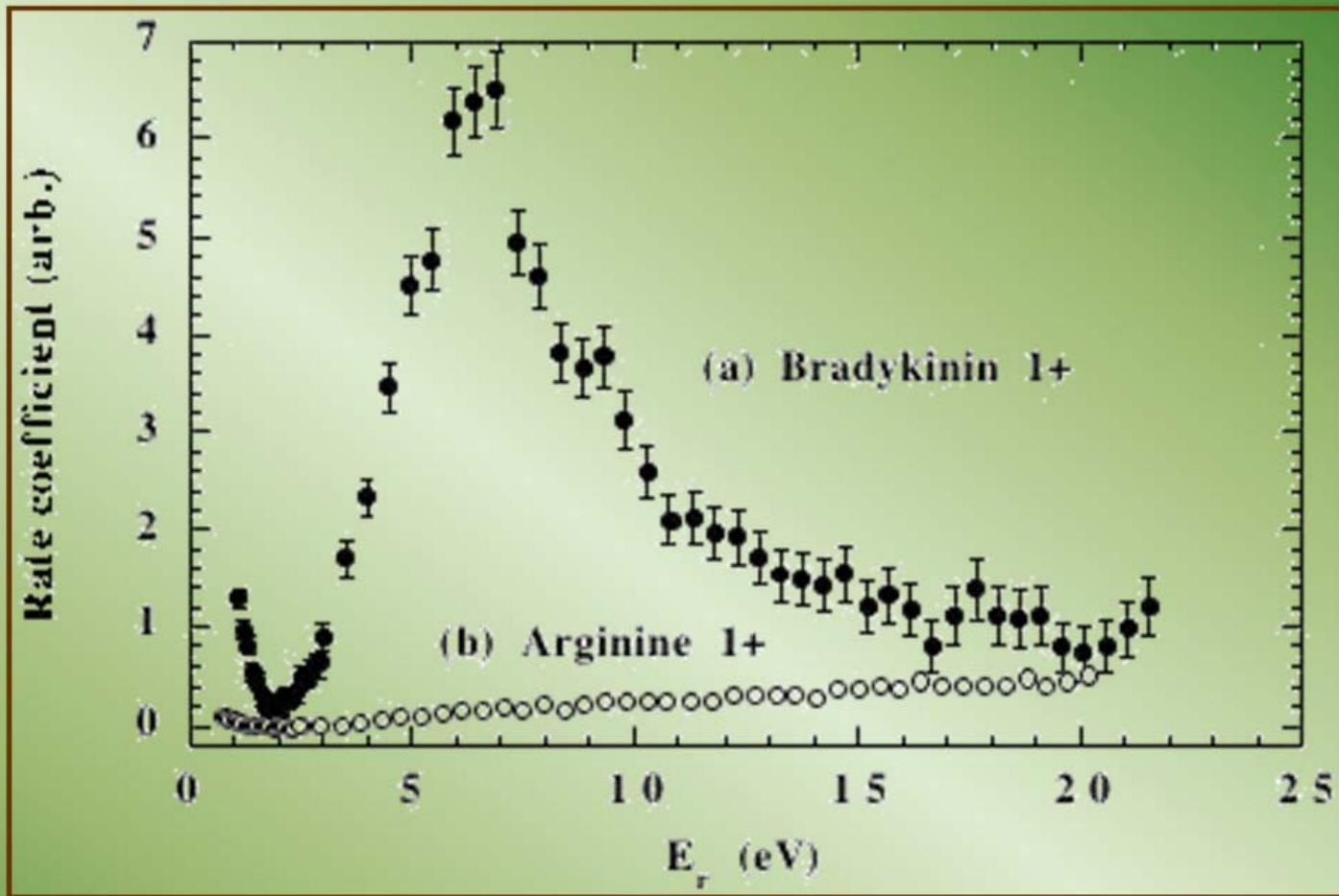
Neutral-particle production rate as a function of the relative energy for singly protonated arginine and bradykinin
