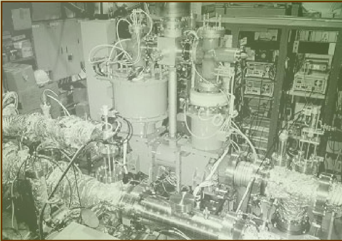
**Photograph of the electron target installed in the KEK electrostatic ring.**
