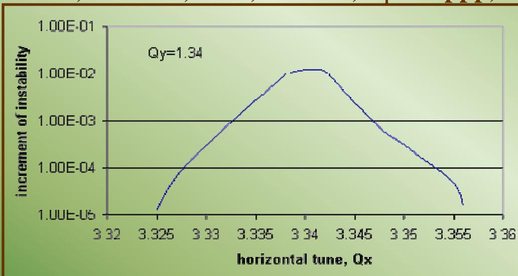
Dependence of the increment of instability on the horizontal tune at  $Q_y=1.34$ ,
