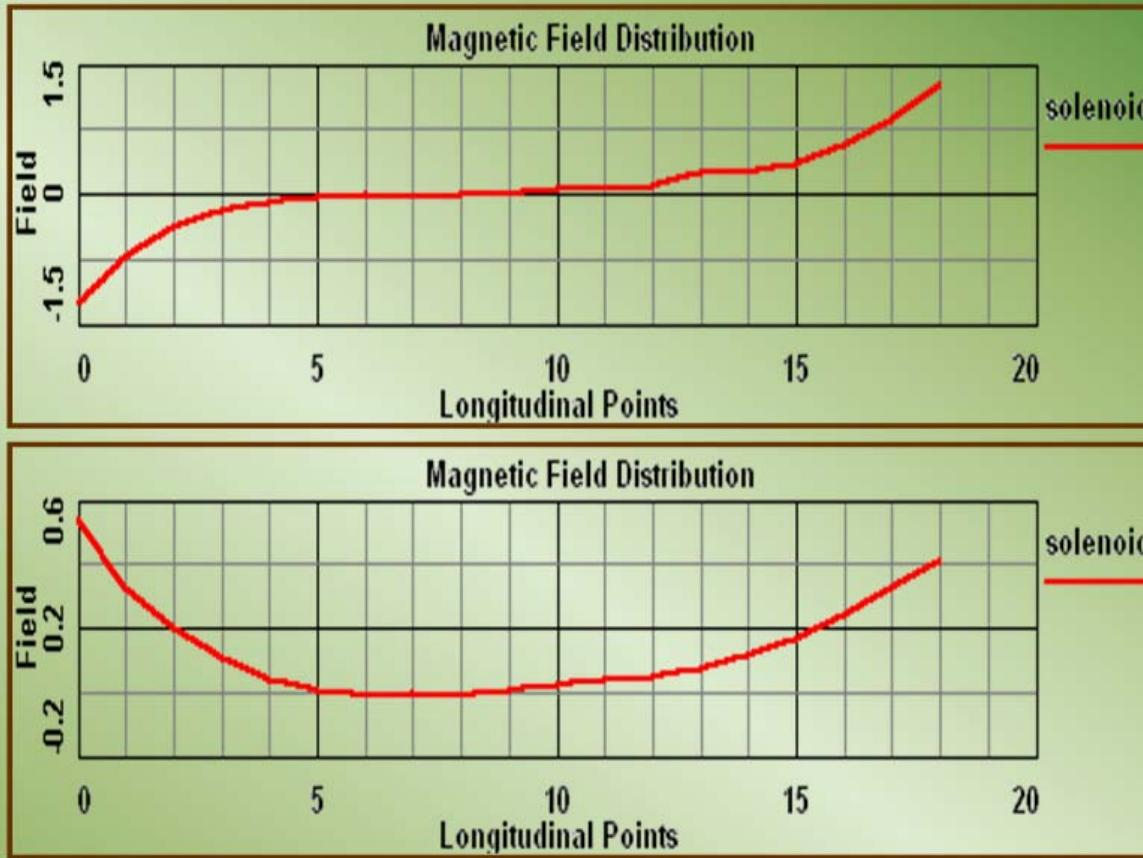
The vertical and horizontal magnetic field for  $B=30$  G.
