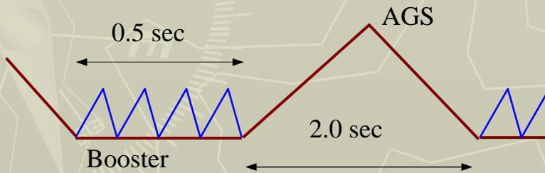
Typical DTL cycle for Protons
