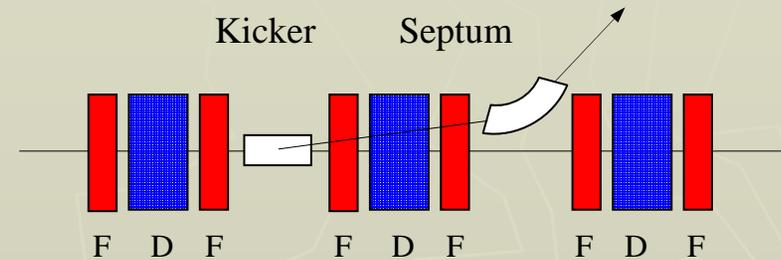
The Kicker field remains constant for the duration of the beam pulse (about 2.6  $\mu$ s), and it is finally reset to zero-value in about 100 ms, to be fired again the next cycle.
