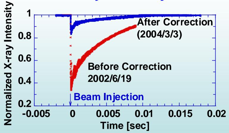
X-ray intensity measured by silicon photodiode in BL39
