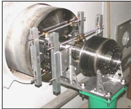
Figure 9: Co-Axial Bellows & Vacuum Clamp Assembly
