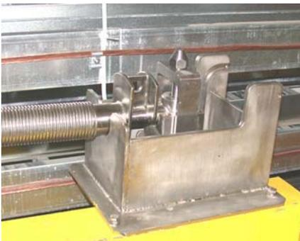
Figure 4: Quick Release Water Coupling
