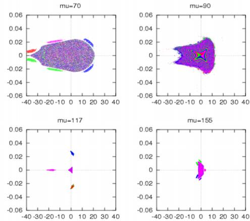
Figure 4 :  $(\delta\varphi, \delta p/p)$  stable areas for phase advances per period equal to  $70^\circ, 90^\circ, 117^\circ$  and  $155^\circ$ .
