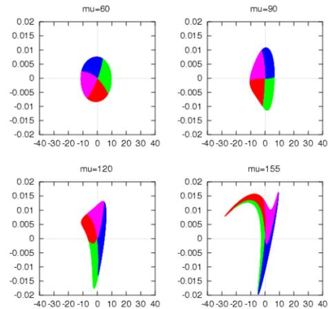
Figure 5 :  $(\delta\varphi, \delta p/p)$  portraits after two cells for a geometrical emittance  $57\pi \text{ mm.mrad}$ , and the phase advance values :  $\mu = 60^\circ, 90^\circ, 120^\circ$  and  $155^\circ$ .
