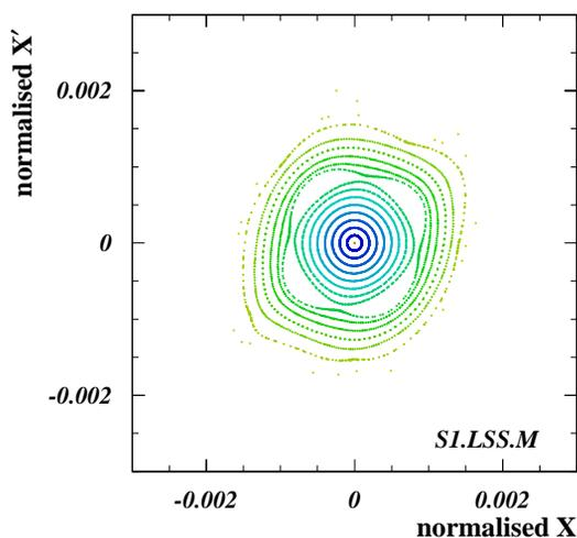
Figure 3: Horizontal phase space in the middle of the first long straight section generated with the MAD program [3] for the full nonlinear ANKA optics model.
