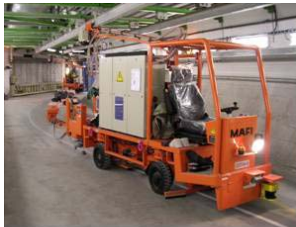
Figure 4: A cryo-dipole transport vehicle follows the guidance line in a bypass tunnel.
