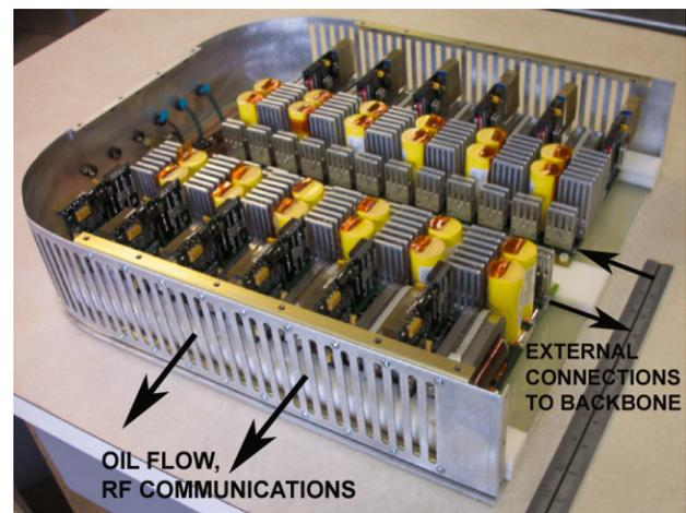
Figure 4: Block Assembly containing 12 Marx Cells.
