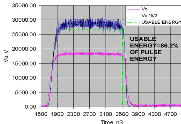
Figure 7: Waveform efficiency.
