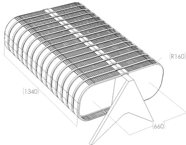
Figure 3: Proposed Marx Modulator. Dimensions in mm.
