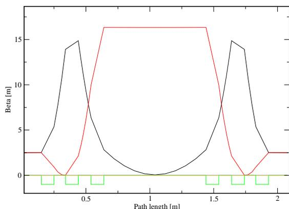
Figure 1: Optics of the matching section between ideal (hard edged) solenoids
