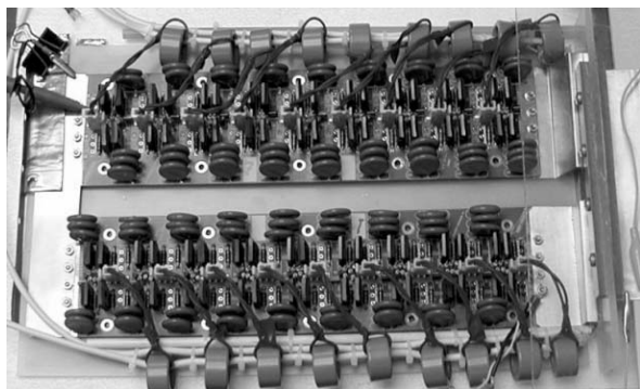
Figure 4: A series/parallel array of 1200 V IGBTs in discrete TO-247 packages makes for a very fast hard switch. This assembly is capable of 11 kV operation, with about 25 ns risetime into a 100 \Omega load.
