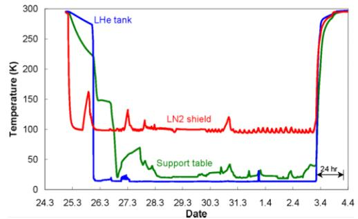
Figure 3: Temperatures of the LN<sub>2</sub> shield, the support table and the dummy helium tank during HOBICAT commissioning. Measurements were made with CLTS sensors which were not fully calibrated at LHe temperatures and therefore bottom out at around 10 K.
