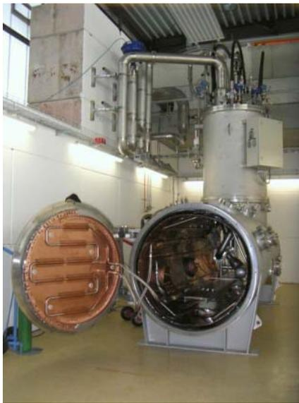
Figure 1: The HOBICAT cryostat and feedbox in the radiation enclosure.
