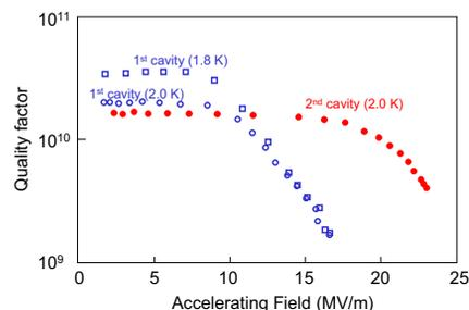
Figure 5: Vertical cavity tests of the HOBICAT cavities at DESY.
