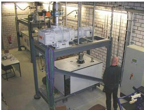
Figure 2: A combination of Leybold RA7001FU roots blowers and Sogevac SV1200 rotary vane pump is used to pump the HOBICAT helium bath to 16 mbar.
