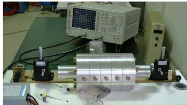
Figure 8: Deflector aluminum prototype and measurement setup.
