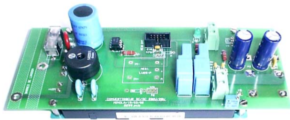
Figure 2: Power supply board.
