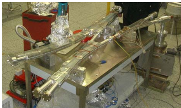
Figure 2: Dipole vacuum chambers under test.
