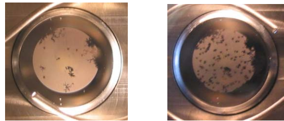
Figure 5: Damaged \text{Cs}_2\text{Te} film on the cathode #60. Photographs were taken on March (left) and May (right) 2004.
