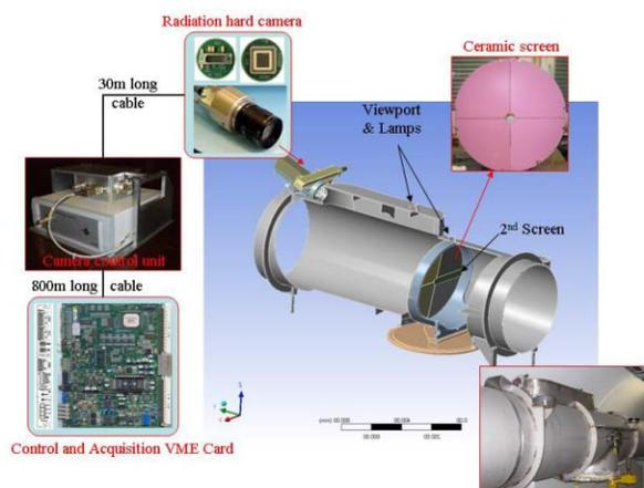
Figure 3: Overview of the BTVDD imaging system
