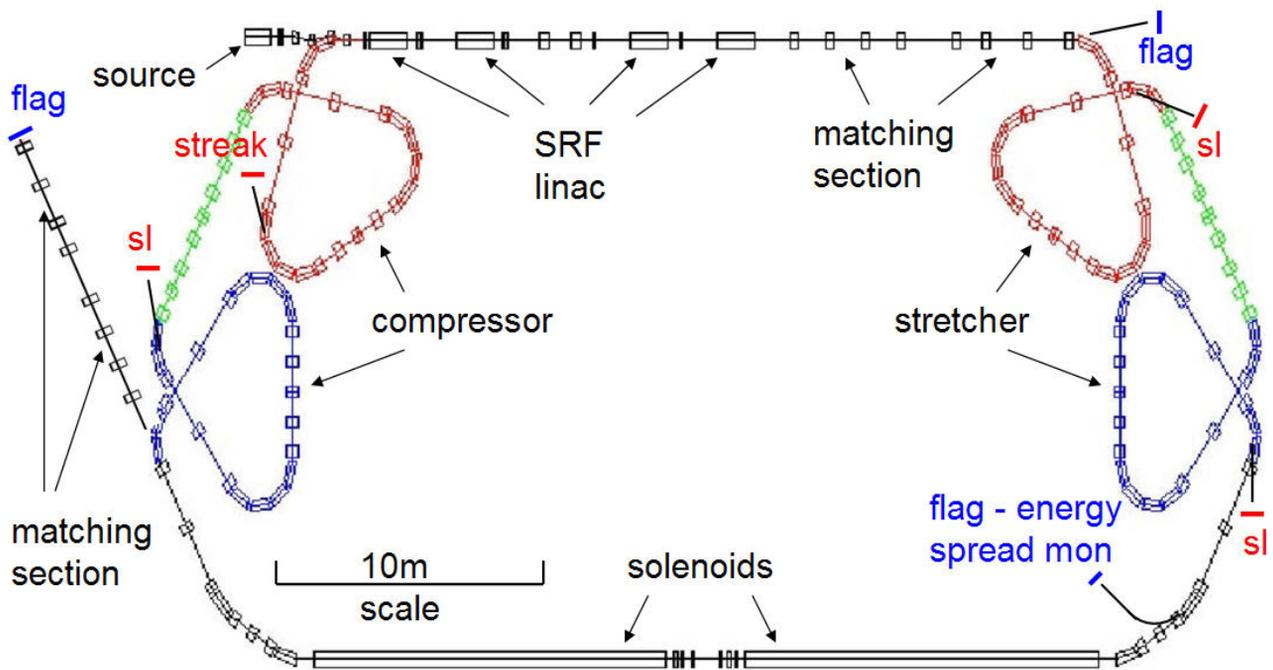
Figure 1: Layout of the RHIC Electron Cooler
