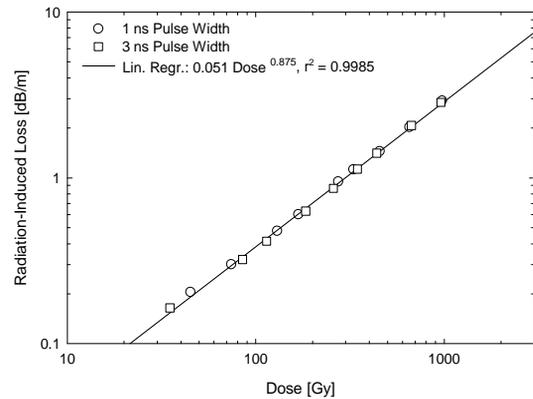
Figure 2: Loss increase with dose of the (Ge+P)-doped MM GI fibre FiberCore N2900107GA during  $^{60}\text{Co}$  gamma irradiation. Measurements were made with the 850 nm multi-mode module of the OTDR and pulse lengths of 1 ns and 3 ns, respectively.
