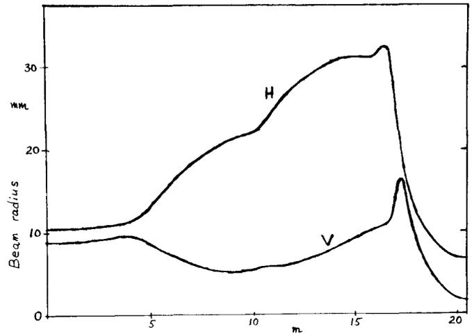
Figure 9 Half axes of uncooled beam with emittance and momentum spread typical for injection.
