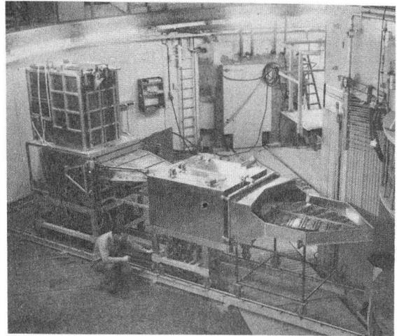
Figure 6 RF system: from left to right amplifier dee cavity tuning section and dee electrode in test chamber.
