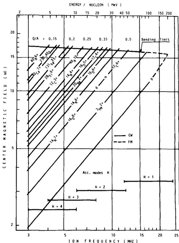
Figure 2 Final ion energies vs ion frequencies and harmonic number. Bending limit is shown.
