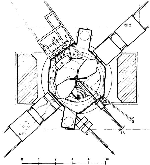
Figure 3 Cyclotron median plan with main components.
