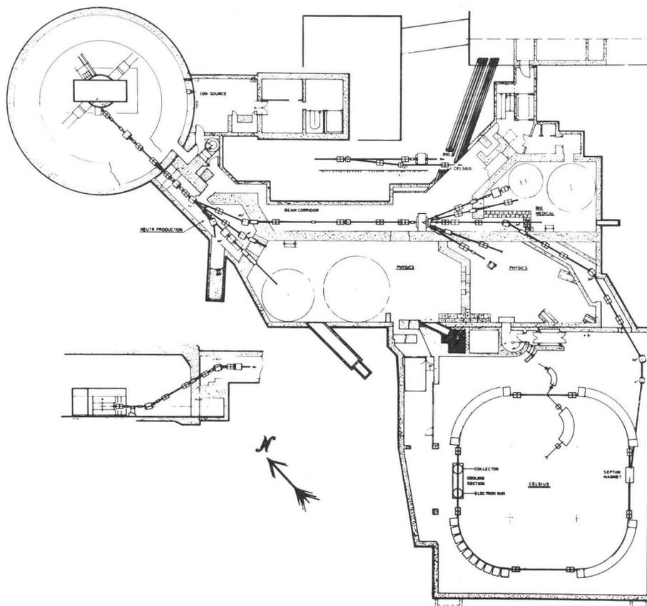
Figure 1 Floor plan of the cyclotron, the CELSIUS ring and the experimental areas.
