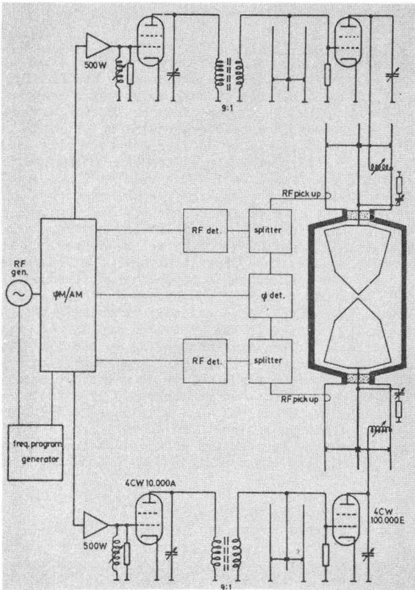
Figure 4 Block diagram of the RF system.
