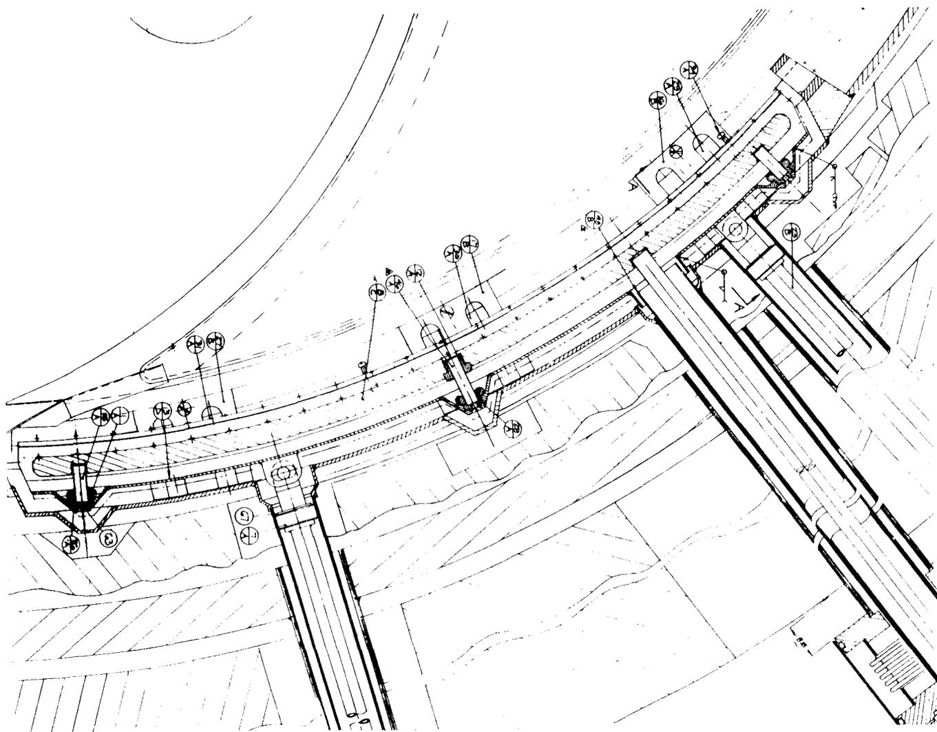
Fig. 1. A section of the K500 median plane showing the region around the second electrostatic deflector, E2.
