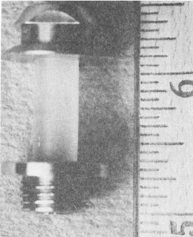
Fig. 2. A photograph of the new plane geometry insulator: sapphire rod soldered to copper buttons and stainless steel end caps. This is the center insulator (tension) for E1. The copper ends are recessed into the end caps. The scale is in inches.
