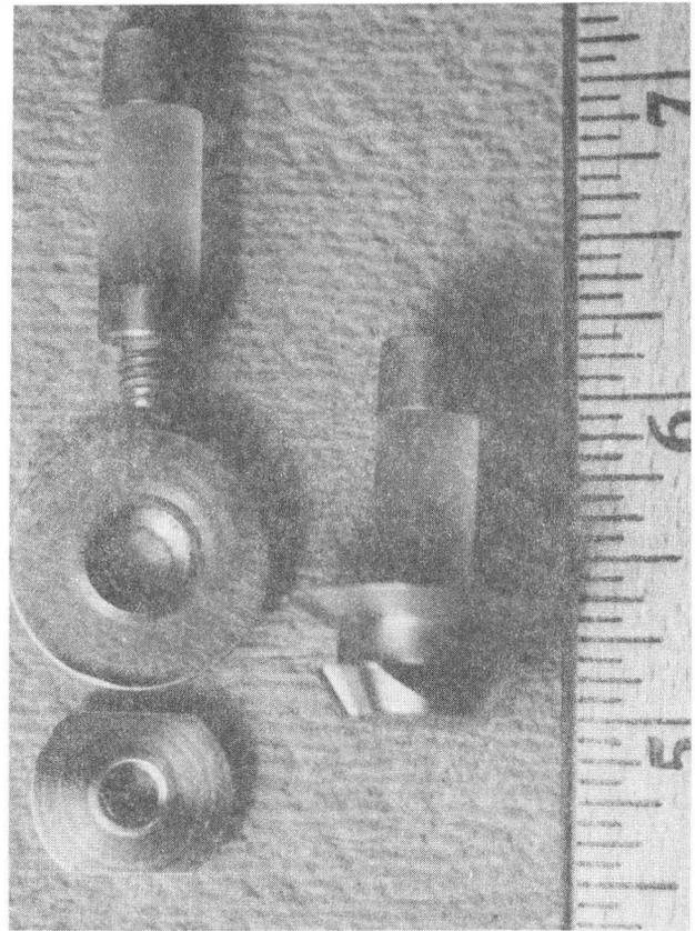
Fig. 3. A photograph similar to figure 2, except of the new end insulators (compression) for E2. Two insulators are shown, one disassembled to show the separate pieces.
