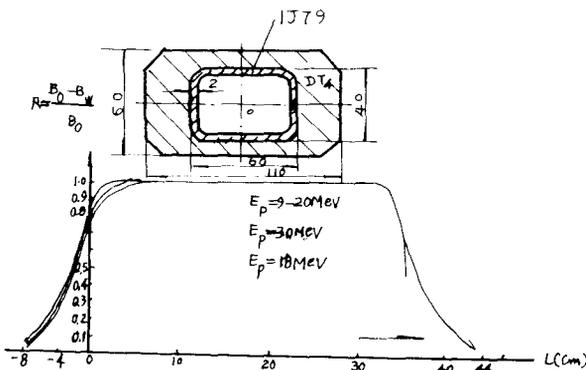
Fig.8 Magnetic shielding coefficient
