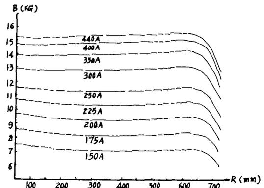
Fig.2 Average fields vs radius for main coil excitation
