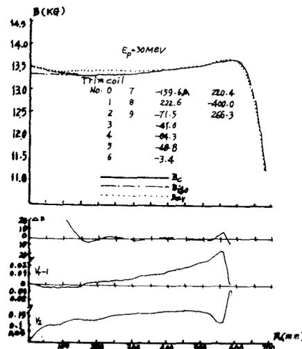
Fig.3 corrected field, field deviation from the isochronous, and  $\nu_r, \nu_z$
