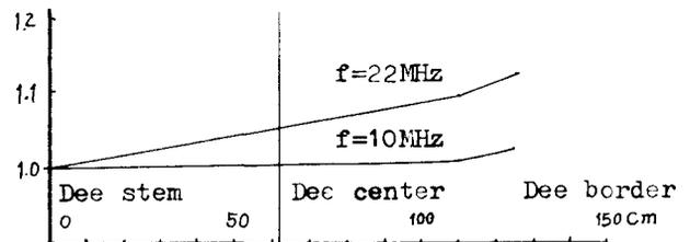
Fig.6 Relative radial voltage distribution along the Dee
