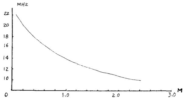
Fig.5 Resonance frequency vs length of resonator
