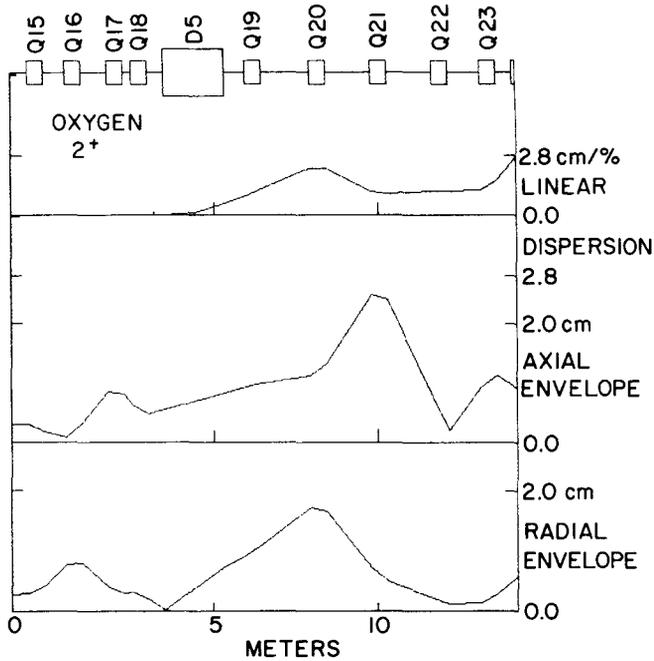
Fig. 4. Plots of linear dispersion, axial envelop, and radial envelop for oxygen 2+ beam to be injected into the K800.
