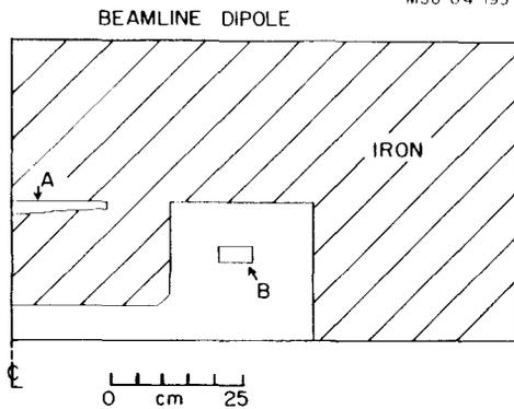
Fig. 5. Upper right quadrant of a cross-section of the 135° dipole. "A" is the tapered "flux guide" (tapered Purcell filter) and "B" is the coil.
