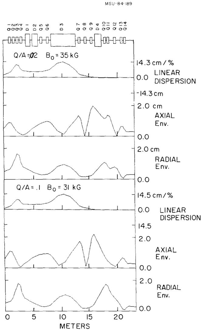
Fig. 2. Plots of linear dispersion, axial envelop, and radial envelop for  $Q/A = .02$ ,  $B_0 = 35$  kG and  $Q/A = .1$ ,  $B_0 = 31$  kG beams from the K500 up to the achromatic double-waist.
