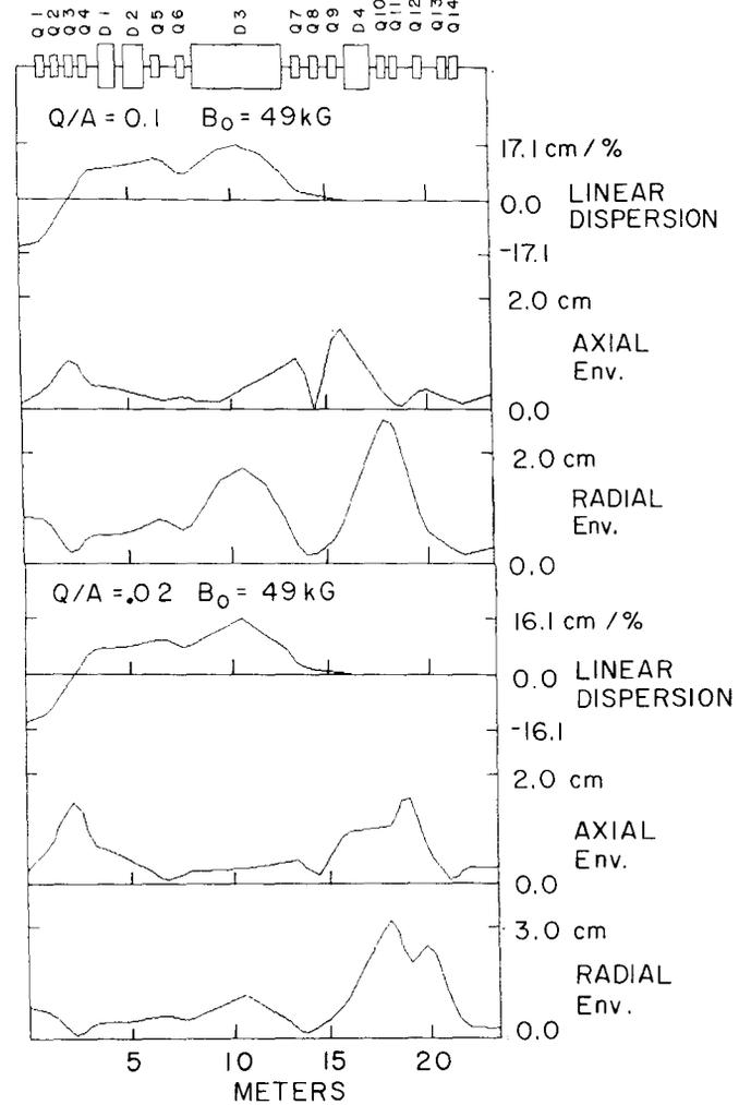
Fig. 3. Plots of linear dispersion, axial envelop, and radial envelop for  $Q/A = .1$ ,  $B_0 = 49$  kG and  $Q/A = .02$ ,  $B_0 = 49$  kG beams from the K500 up to the achromatic double-waist.
