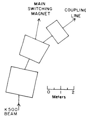
Fig. 6. Scaled plan view of initial beam switching area. Beam comes from the K500 cyclotron, bends 21° in the first dipole, and is switched into the injection line (additional 16° bend) or toward the main switchyard magnet by the second dipole (dipole is reversed and bends the beam -10°).
