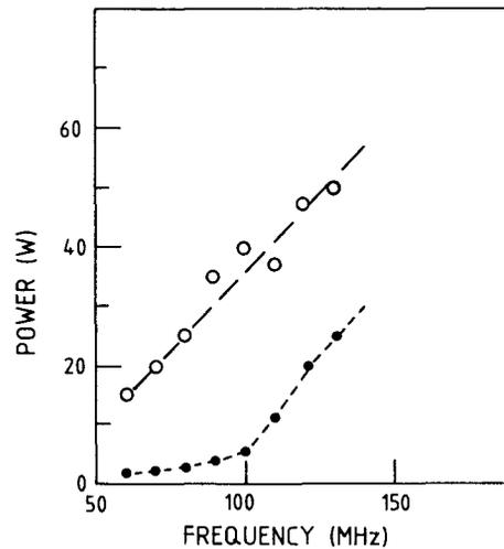
Fig. 9 The pulsed power required to breakthrough the multipactoring is shown by the upper curve. The lower curve shows where the multipactoring starts again as the power level is reduced. These tests were limited by the output of the power amplifier but indicate that operation at high frequencies is possible above about 80 watts.
