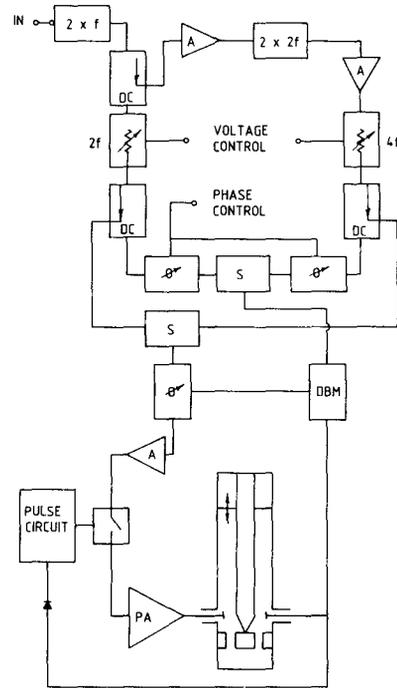
Fig. 7 The rf drive modulator showing the generation of the 2f and 4f signals to drive the power amplifier and to provide reference signals to stabilize the phase.
