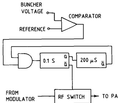
Fig. 8 The pulsing circuit for multipactor breakthrough. With no buncher voltage the rf is pulsed on for 200  $\mu$ s every 0.1 s. If the buncher voltage rises beyond the multipactor level, which is only a few watts, the comparator signal to the "And" gate holds the rf switch on continuously.
