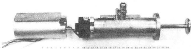
Fig. 3 Photograph of the rf drive capacitor assembly removed from the resonator.
