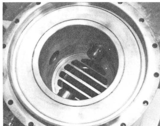
Fig. 4 A view into the copper vacuum cavity. The "noses" of the drift tube assembly can be seen on either side and the vacuum port grill on the bottom.
