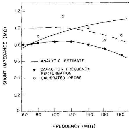
Fig. 6 The shunt impedance vs frequency measured by two methods compared with an analytic estimate.
