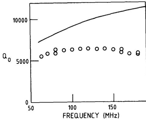
Fig. 5 The measured  $Q$  of the resonator compared with the analytic estimate.
