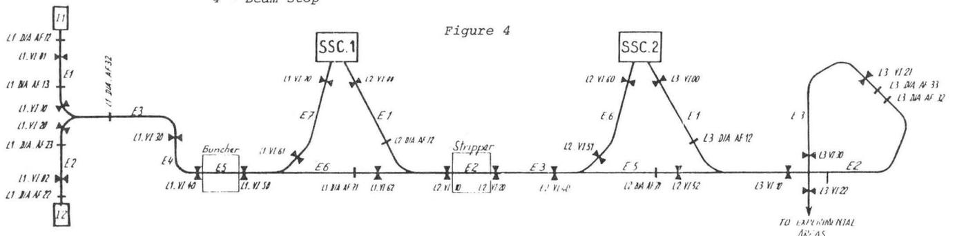
The conductance between I1 and the beam-line is very low, so the I1 pumping system does not contribute to the line vacuum. Then two phenomena act together : the distributed desorption and the localized one. The last one gives a linear pressure distribution (see Fig. 5). The average pressure between pump 1 and FC, and the one between FC and I1 have to be separate. So the average pressure between I1 and A is given by :
