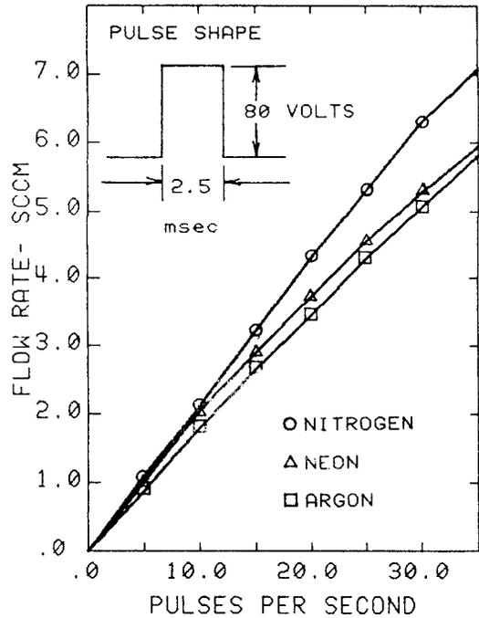
Fig. 7. Performance of a Veeco piezoelectric leak valve for selected gases, when drive by a variable pulse rate, square wave voltage signal as given, at an inlet gas pressure of 1 psi above atmosphere.
