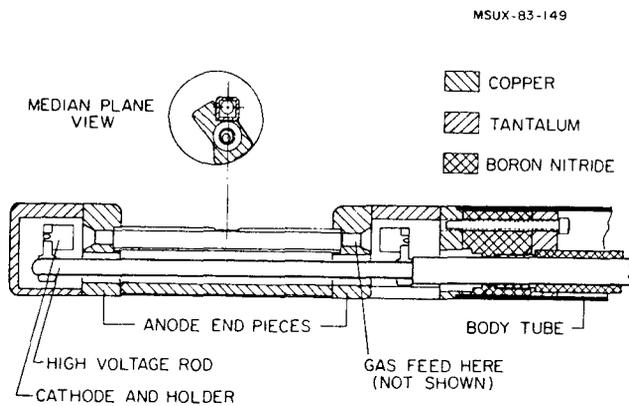
Fig. 1. The K-500 cyclotron heavy-ion PIG source.
