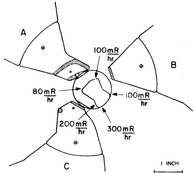
Fig. 2. Activation of the cyclotron central region, after a 56 h lifetime source for  $N^{4+}$  at a final beam energy of 30 MeV/n. Stripping to  $N^{5+}$ , with a subsequent bombardment of the central region, is thought to cause this activation.
