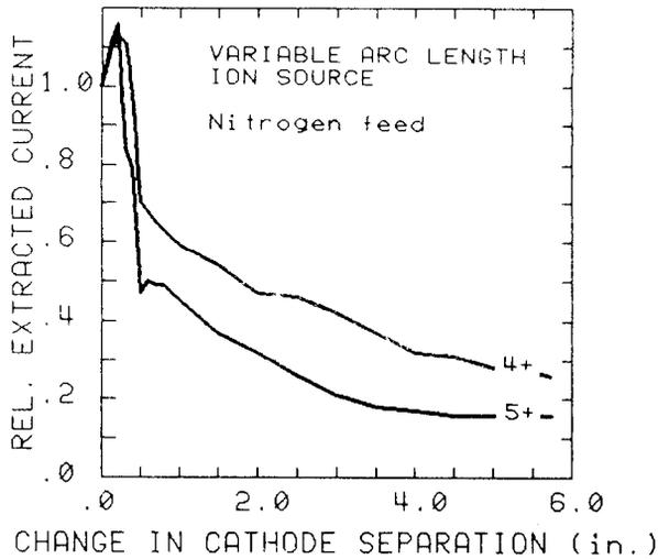
Fig. 6. Variation of  $N^{4+}$  and  $N^{5+}$  currents from the variable arc length PIG source, with the change in cathode separation from an initial separation of 4 in.
