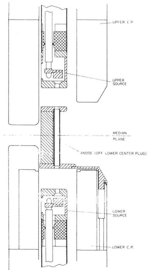
Fig. 5. Experimental source configuration used to study ion production as a function of cathode separation (see text).
