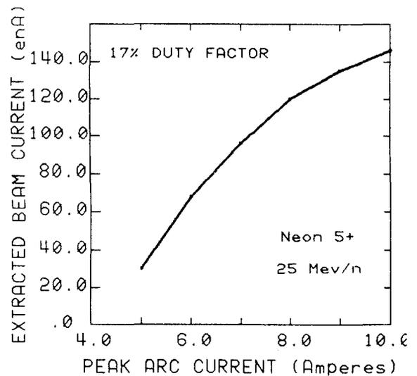
Fig. 3. Dependence of beam current with arc current for Ne<sup>5+</sup> at a 17% duty factor.
