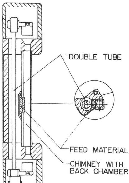
Fig. 4. Modifications to the basic source design to accommodate solid feed via the back-bombardment sputtering process.
