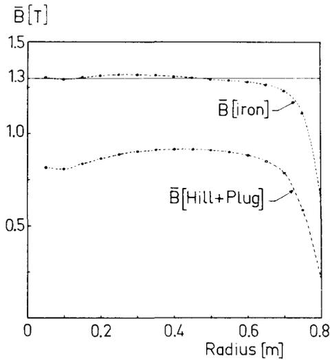
Fig.4 - Contributions to the mean induction, lower curve : hills and central plug ; upper curve in dotted line hills + plug + valleys continuous line : expected  $B_{iron}(r)$ .
