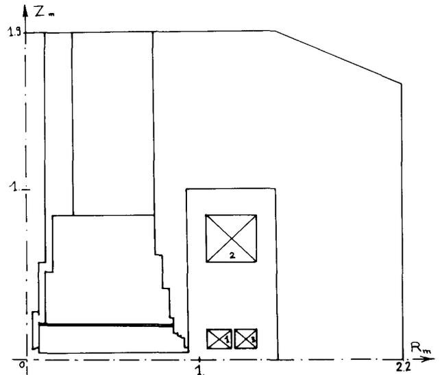
Fig. 1 - Sectional view of a quarter of the IPN Orsay project magnet showing the uncommon main coil cross section. Part.1, creates the radial gradient; parts 2 and 3 in series flat fields.
