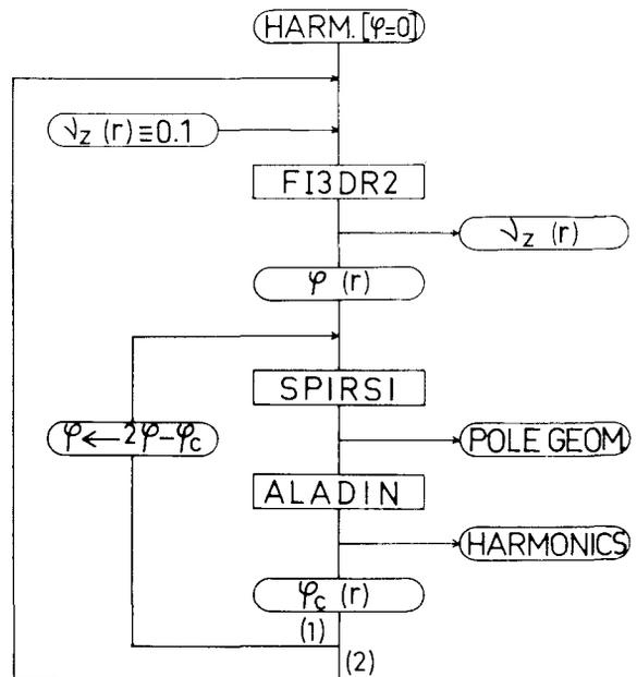
Fig.7 - Schematic organization of the computer codes for the treatment of the second part of the pole geometry determination method which delivers the spiraling law. A two steps iteration is necessary in which an enhanced convergence process is introduced.
