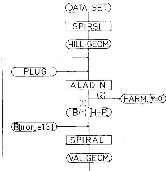
Fig.6 - Schematic organization of the computer codes for the treatment of the first part of the pole geometry determination method. The goal is the valley profile when  $g_h$  and  $B_{iron}(r)$  are given. The method is applied to a fictive right-sectored machine.
