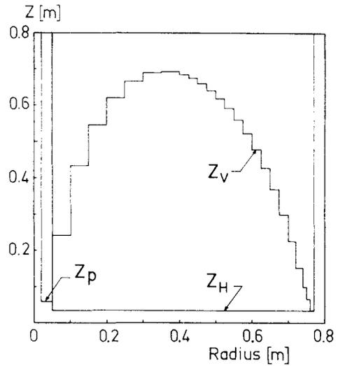
Fig.5 - Valley profile calculated by "SPIRAL" for the starting right-sectored machine, in the case mentioned in the text as an example.
