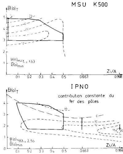
Fig.2 - Trim coil consumed power comparison between MSU-K 500 and IPN-Orsay project.
