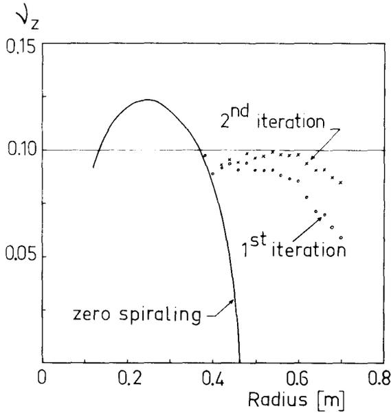
Fig.8 -  $v_z$  as a function of the radius in the case of the machine treated as an example (Hagedoorn-Verster formula).
