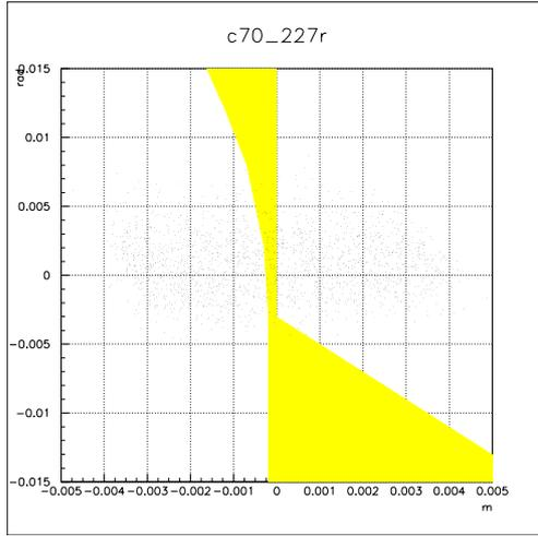
Figure 1: Horizontal phase space plot of 2 turns at the entry of the septum. The septum is shown with its apparent thickness as the yellow filled surface. The septum is angularly displaced in order to obtain an optimum extraction efficiency.
