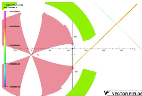
Figure 4: Tracking simulation in the *TOSCA* field for the 70 MeV extraction, stripper to switching.
