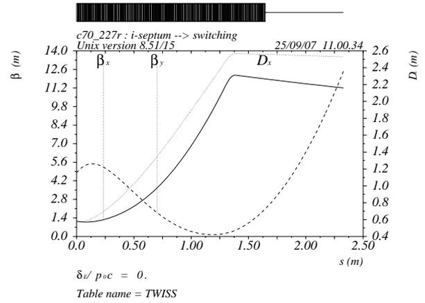
Figure 2: *MAD* plot of the optics between the septum entry and the switching magnet.
