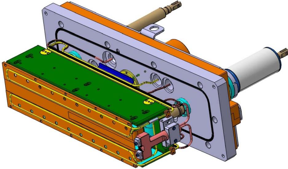
Figure 3: General view of the C70 deflector, the beam entry being in the foreground.
