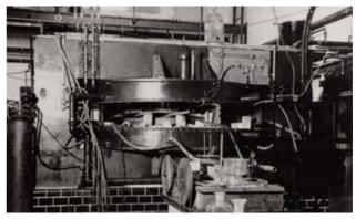
Figure 1: The Niels Bohr Institute cyclotron.
