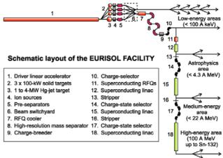
Figure 11: Schematic layout of the EURISOL project.
