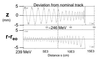
Figure 5: Track of an accelerated particle relative to the reference track starting at 239 MeV. The vertical deviation (top) and the horizontal deviation (bottom) are shown as a function of covered distance. The horizontal scale represents a distance covering ~30 turns.
