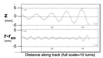
Figure 4: Track of a particle relative to the 246 MeV equilibrium orbit in the vertical plane (top) and in the horizontal plane (bottom).
