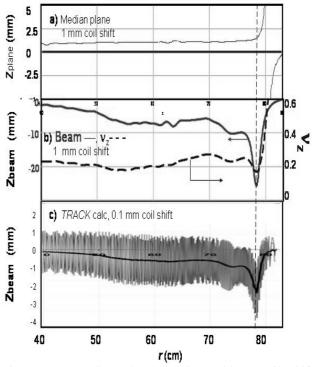
Figure 1: a) Median plane position with a coil shift  $\delta = 1$  mm. b) beam position from eq (4) and  $v_z$ , c) *TRACK* results with  $\delta = 0.1$  mm for different particle starting conditions. The dashed line at r=78 cm is at minimum  $v_z$ .
