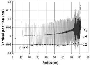
Figure 2: Vertical particle position as a function of radius when the coil is tilted 0.38 mrad. Dark line: particle starts at centre of iron gap, grey line: particle starts 1 mm above centre. Dashed line:  $v_z$ .
