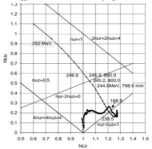
Figure 3: Plot of the betratron frequencies and resonances in the measured field of COMET. Some key energies and average orbit radii are indicated.
