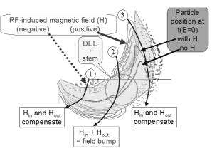
Figure 6: Three numbered particle tracks crossing the Dee and its H(t) field. The particle positions at t(E=0) with and without H(t) field are shown.
