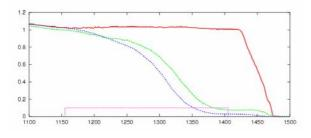
Figure 6: Normalised beam current as a function of the radius for a beam phase shift of  $40^\circ$ : red = no voltage, green  $\approx 370$ V, blue  $\approx 500$  V.
