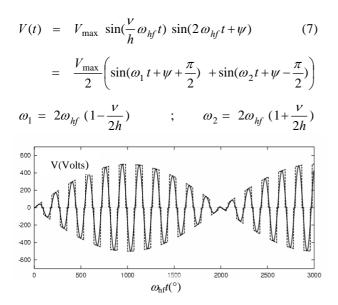
Figure 1: Ideal and realistic potential signals  $V(\omega_{hf})$ .
