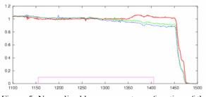
Figure 5: Normalised beam current as a function of the radius (isochronised) : red = no voltage, green  $\approx$  370V, blue  $\approx$  500 V, pink=position of electrodes.
