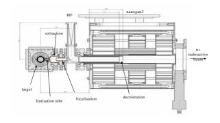
Figure 5: The nanonake configuration for alcali elements.
