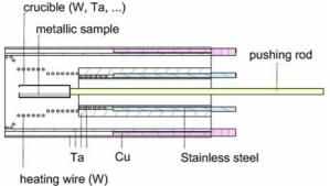
Figure 1: Sketch of the high temperature oven.
